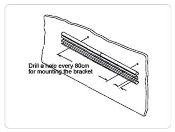
1. Place a horizontal line on the wall (the bottom of the handrail is 80-85CM from the ground). The bracket is fixed to the wall. and the position of the bracket is fixed from the distance of 25cm from the frame of the two sides, and is evenly distributed around 80cm. Measure the actual length between the door frames, and then subtract 16cm (two elbow lengths ) from the actual length to cut the aluminum alloy profile.
