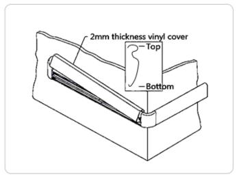
Retain the vinyl cover and trim the interface between the ends of the cover and the elbow with a file.
