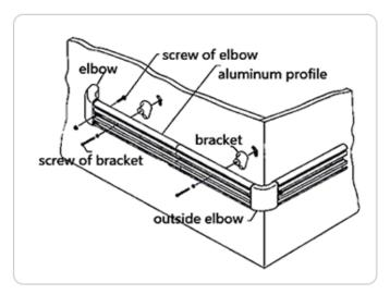
3. After fixing the aluminum profile, measure the distance between the elbows on both sides, and then cut the vinyl cover. Before the cutting of the vinyl cover, the two ends of the material should be trimmed first.
